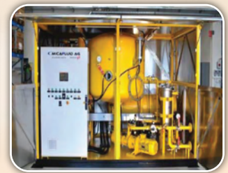
Transformer Oil Centrifuging Machine
